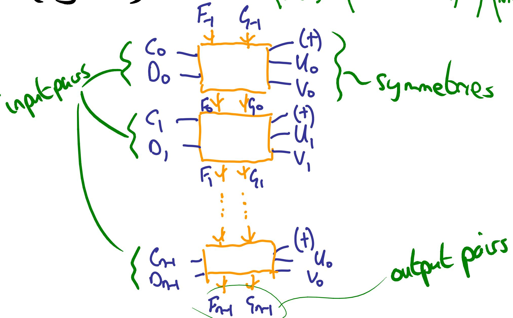
Pair Recursion for  $\{1, -1\}$  arrays  $M_j = \begin{pmatrix} C_j(y_j) & D_j^+(y_j) \\ D_j(y_j) & C_j^+(y_j) \end{pmatrix}$
