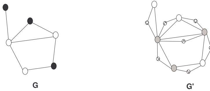
Figure 2.1: On the left hand side, the black nodes indicate the independent set. On the right hand side, small nodes are the nodes added to G to construct G' . The grey nodes indicate a minimum dominating set of G'
