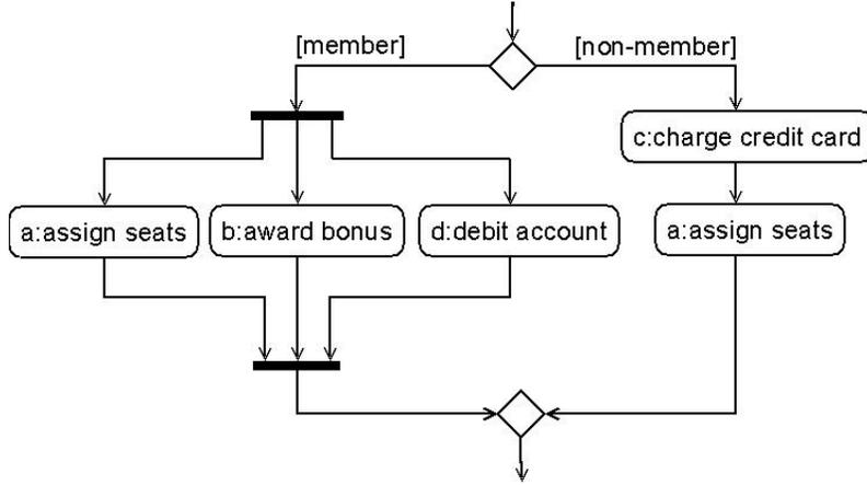
Figure 1: A UML activity diagram for ordering seats
