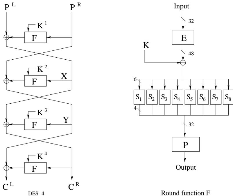
We can now describe the whole encryption algorithm as a system of equations. The straightforward way will be to let each output bit of each S-box be a function of the input bits. Since the four bits output from the same S-box share the same input, it is more efficient to group these four equations into one, and make one configuration list for the input and output variables of the S-box. One equation in our system will thus have the form
