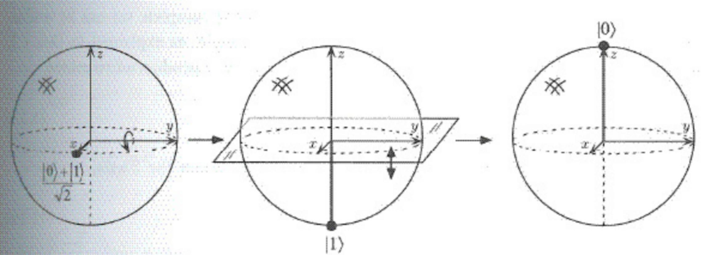
Figure 1.4. Visualization of the Hadamard gate on the Bloch sphere, acting on the input state  $(|0\rangle + |1\rangle)/\sqrt{2}$ .
