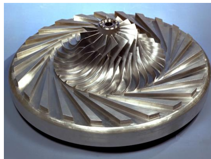
FIGURE 2.13: Centrifugal compressor impeller inside a wedge diffuser – Photo: NASA, U.S. Government (public domain)
