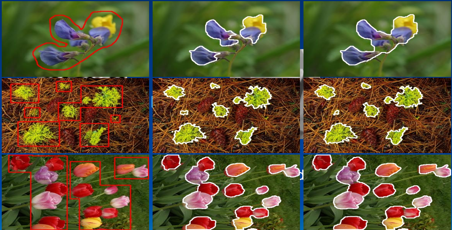
Fig. 9 The comparison between the proposed method based on MPC-GAC by k-means learning and the GrabCut method based on MAP-MRF by GMM estimating. Columns (from left to right): the original image and the initial curve, the results by the proposed method, the result by the GrabCut method.
