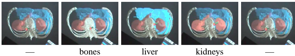
Figure 1.11: Several snapshots from a video which was taken through a session where the user moved a 3D pointing device across a 3D dataset of a human chest in a virtual environment. Visual object high-lighting reflects the current 3D position of the 3D pointing device which is very useful to efficiently position the device in 3D space during object selection.
