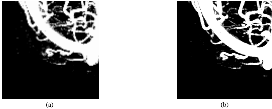
Figure 1: MIP with a) shear-warp projection with nearest neighbor interpolation b) ray casting and trilinear interpolation.
